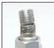
Galvanic corrosion causes TPMS failures.
